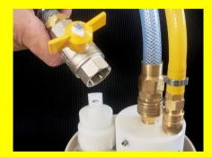
Connect the Breather Hose to BBA. The hose should be used to make sure any water pushed out of the pipe is vented onto the pavement so it drains away from the meter box. The valve on the end should be closed at the start
