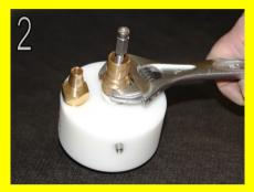
Remove the brass plug connector that the Outlet hose connects to and fit the NRV key in its place with PTFE tape on the thread and tighten. It is important thread does not leak under pressure.
