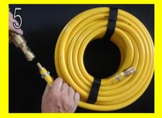
Connect the Inlet Extension Hose to the Inlet Hose and roll out to POE. Make sure the Drive flow is turned off on the Ferret and connect the Inlet Extension Hose to the inlet port on the front of the Ferret.
