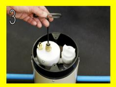
Remove meter or plug from the manifold, check the large "O" ring is correctly located and then fit the Adapter into the manifold and tighten Use the alan key to screw the NRV key down, do not over tighten.
