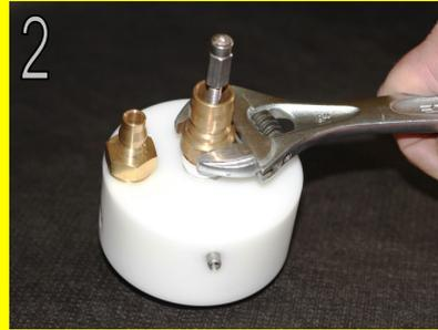
2 Remove the brass plug connector that the Outlet hose connects to and fit the NRV key in its place with PTFE tape on the thread and tighten. It is important thread does not leak under pressure.
