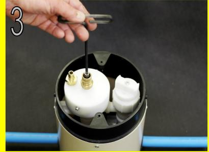
3 Remove meter or plug from the manifold, check the large "O" ring is correctly located and then fit the Adapter into the manifold and tighten Use the alan key to screw the NRV key down, do not over tighten.
