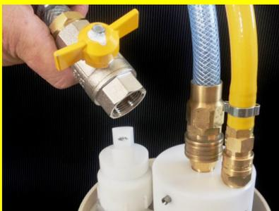
4 Connect the Breather Hose to BBA. The hose should be used to make sure any water pushed out of the pipe is vented onto the pavement so it drains away from the meter box. The valve on the end should be closed at the start
