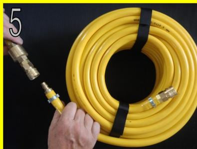
5 Connect the Inlet Extension Hose to the Inlet Hose and roll out to POE. Make sure the Drive flow is turned off on the Ferret and connect the Inlet Extension Hose to the inlet port on the front of the Ferret.
