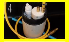
Connect the yellow Inlet Hose to the adapter and turn on the stopcock and check that there are no leaks from the adapter. Then connect the other end of Inlet Hose to Ferret. (Note - The end of the inlet hose with the NRV fitted should be connected to the Ferret)
