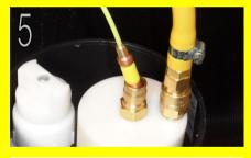
Use the Head Size and Bend Prover, as shown, to establish if a size 1 or size 2 Ferret Head should be used and to test for 90 degree bends and lead gripper joints that might damage the Ferret cord. Then remove the Head Size and Bend Prover tool.
