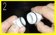
Remove the Non Return Valve mechanism and small "O" ring from the housing and retain for re-fitting later. Then refit the housing without the Non Return valve mechanism back into the meter manifold.
