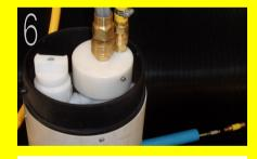
Feed the Cord from the Ferret through the Outlet Hose and then attach the selected Ferret Head. Then manually push approximately 1m of cord through the connection on the Adapter. Connect the Outlet Hose to Adapter and the Ferret is ready for operation.
