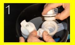
Remove water meter or manifold plug. Then remove the Non Return Valve housing and small "O" ring from the meter manifold. Ensure that the large "O" ring on the water meter manifold is removed and retained for re-fitting later.
