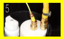
Use the Head Size and Bend Prover, as shown, to establish if a size 1 or size 2 Ferret Head should be used and to test for 90 degree bends and lead gripper joints that might damage the Ferret cord. Then remove the Head Size and Bend Prover tool.
