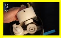
Before fitting the adapter check that the large "O" ring is correctly located. Then screw the male threaded adapter into the female thread in the meter manifold. Tighten the adapter with a meter fitting key.
