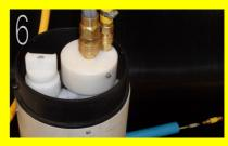
Feed the Cord from the Ferret through the Outlet Hose and then attach the selected Ferret Head. Then manually push approximately 1m of cord through the connection on the Adapter. Connect the Outlet Hose to Adapter and the Ferret is ready for operation.
