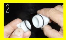
Remove the Non Return Valve mechanism and small "O" ring from the housing and retain for re-fitting later. Then refit the housing without the Non Return valve mechanism back into the meter manifold.
