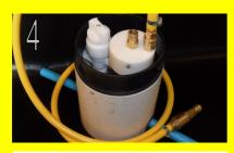
Connect the yellow Inlet Hose to the adapter and turn on the stopcock and check that there are no leaks from the adapter. Then connect the other end of Inlet Hose to Ferret. (Note - The end of the inlet hose with the NRV fitted should be connected to the Ferret)
